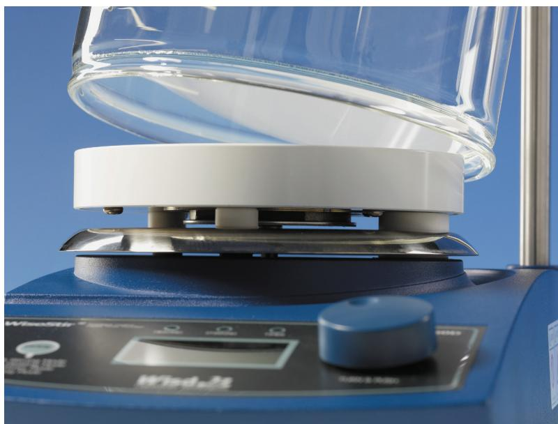
The stirring beakers match with all common hotplates and magnetic stirrers with round stirring plate Ø145 mm and Ø165 mm (such as from witeg®, IKA®, Heidolph®, CAT® etc.)
