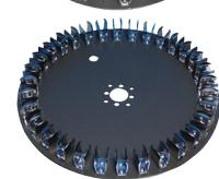
Rotator disc for 32x 1.5ml conical/centrifuge tubes
