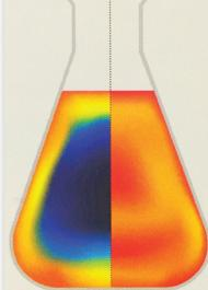
In the Microjet autoclave the thermal energy required for sterilization is supplied directly to the medium. Microwaves from the bottom of the chamber are used as energy source so that the heating of the medium is immediate and uniform.
