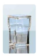
For 10 microscope slides 76 x 26 mm. Note: Do not clean staining dishes and staining jars at temperatures above  $60\,^{\circ}\text{C}$  (glass corrosion is possible).
