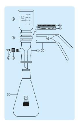
The DURAN® PTFE Adapter combines the ground joint NS 45/40 of the filtering apparatus with the GL 45 screw thread of the DURAN® laboratory bottles. Product benefits: The adapter allows the filtrate to be directly collected in a DURAN® GL 45 laboratory bottle which reduces the risk of contamination. Note: As a vacuum is generated within the bottle during filtration, the use of DURAN® pressure plus+ bottles is highly recommended.
