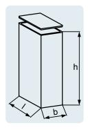
The precise grinding of the glass plate and base vessel enables a very tight seal.
