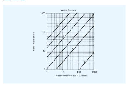
Water flow rate through filter discs of various porosities as a function of pressure differential. For filter discs with  $\emptyset$  30 mm
