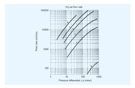
Air flow rate through filter discs of various porosities as a function of pressure differential. For filter discs with Ø 30 mm
