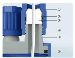
Schematic diagram of GL 45 connection system
